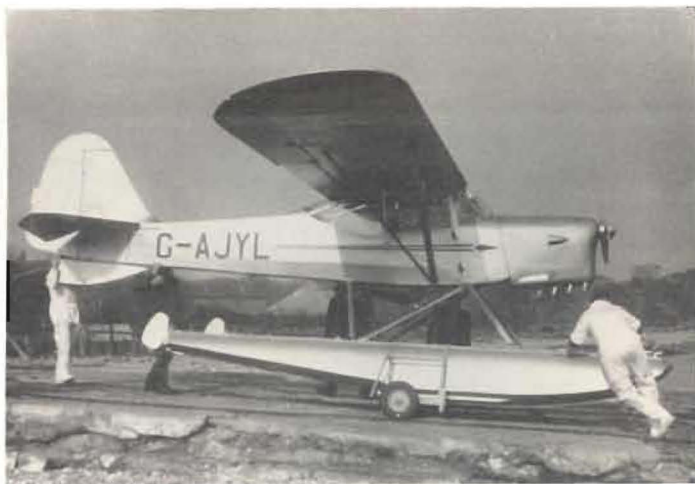
The floatplane being taken down the slipway on its beaching trolleys
